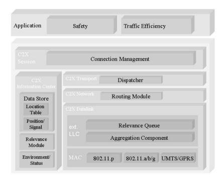
Fig. 2. OpenWAVE Engine Software Architecture
